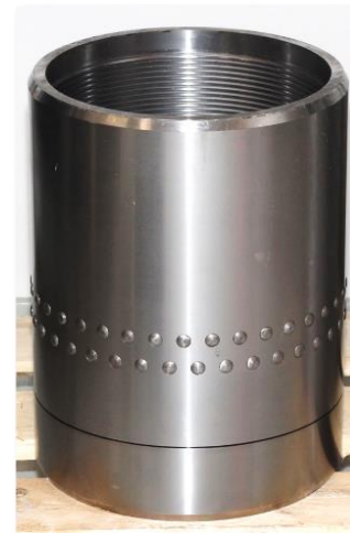
Figure 1. The flexible coupling is designed to allow thermal expansion of casings at 12 m intervals. The figure shows one of the prototypes (for 9 5/8" casing) of the FC that was built and tested in the Horizon 2020 project GeoWell.
